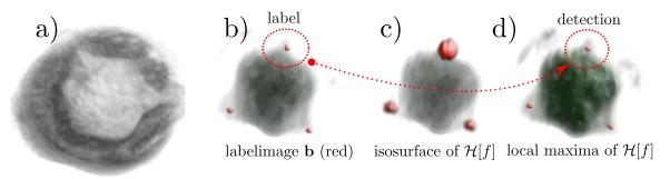
**Fig. 4.** a) 3D rendering of an airborne pollen. b) Labels (here: 3 voxel have been set to 1, all others to 0) are indicating the center of the porates and are used for training and evaluation. c) Isosurface showing the response of the Bessel Filter. d) Local maxima of the responses. The porates are localized very precisely.
